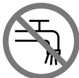
According to the applicable regulations, the appliance must never be used on the drinking water network without a system separator. Use a separator as per IEC 61770 Type BA. Water flowing through a system separator is considered not drinkable.
